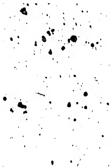
FIG. 2. Unetched Cross Section of Cerium Steel. \times 100 .
