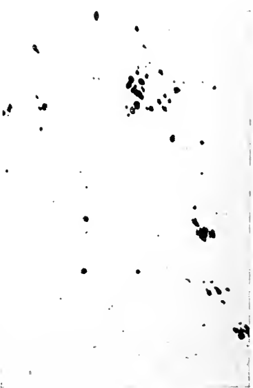
FIG. 5. Unetched Cross Section Chromium-cerium Steel. \times 100 .
