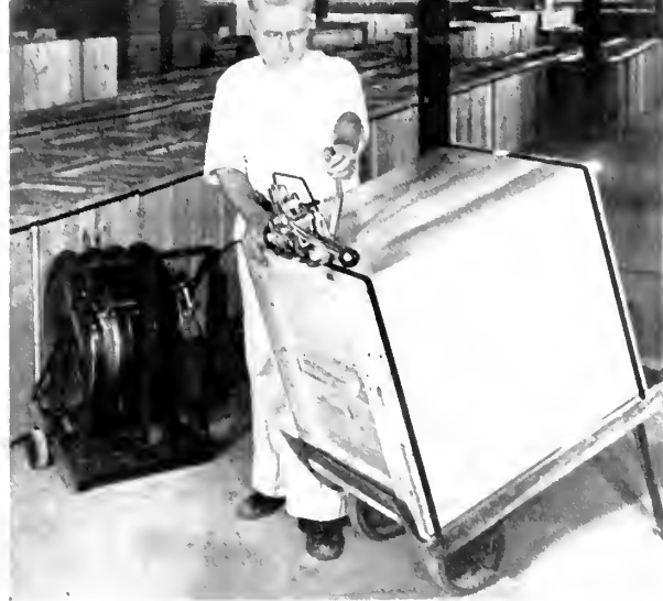
Above, left: Paper, which will be printed into Chinese money, is steel strapped into wooden cases.
