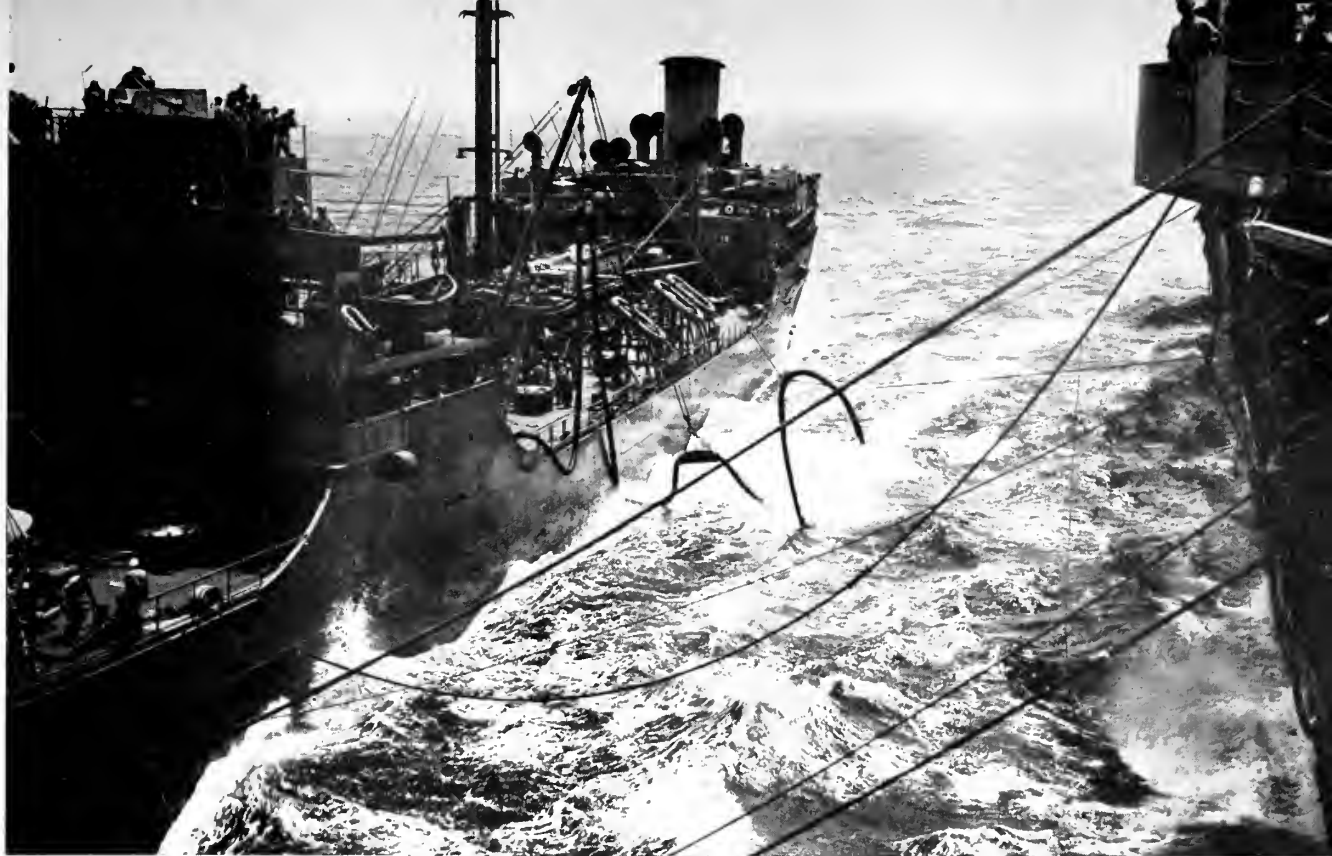
In wartime, battle fleet units were often refueled while under way at sea. Here a Navy tanker is passing hose to a carrier. Under like conditions some Standard of California tankers fueled warships on convoy duty in the Atlantic. (Official U. S. Navy Photo)
