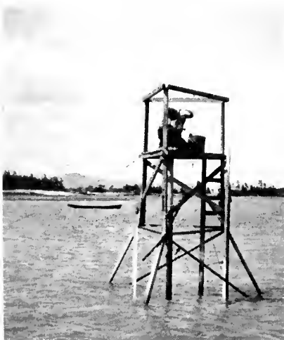
A tide gage. This consists of a staff gage, visible in the picture, and an automatic recording gage by which the height of the tide is measured.
