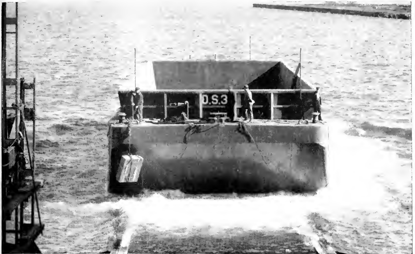
One of 12 barges built for the City of New York goes down the ways at Bethlehem's Staten Island Yard.
