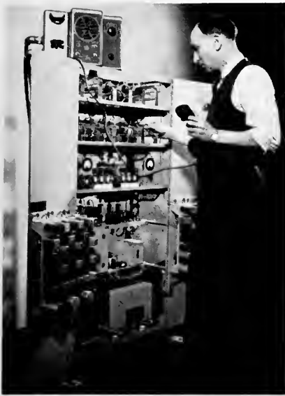
The new 75-watt automatic radiotelephone with remote control unit. Shown receiving its final laboratory check.
