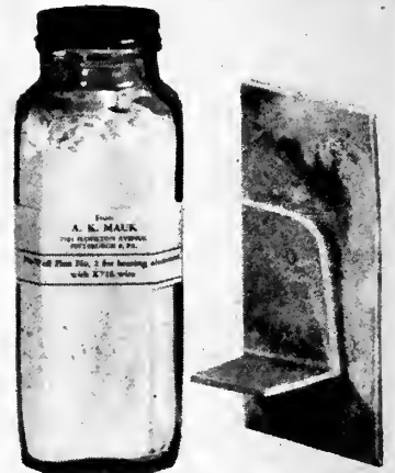
Illustration shows two pieces of aluminum brazed with new Mauk flux.
