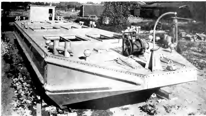
A barge designed for dry cargo only and very shallow waterways. Bow, stern and sides are raked. This type has a crew's house and rudder control. View of assembled barge, showing deck.
