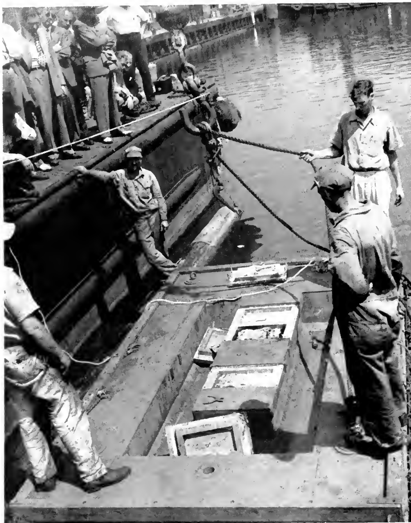
Stowage compartments are opened after drop tests to examine equipment and provisions specified to be aboard life rafts by Coast Guard regulations.
