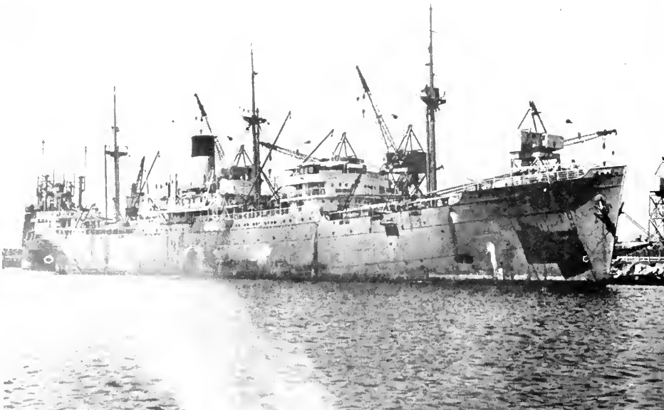
Fig. 22. Motor vessel Poelau Laut, tied up at Bethlehem Steel Company's San Pedro Yard, for repairs. This ship, which was built in Amsterdam, Holland, in 1929, is a three-deck combination freighter and passenger vessel 535 feet long with a beam of 65 ft. It is powered with an 8000 hp Sulzer diesel engine, the largest of its type and the third largest diesel engine afloat.
