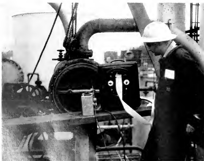
Electronic recorder, 1/2" probe with long flexible cable and sample tube with perforations used for demonstration. Record of tube defect is shown on strip chart. Bulb to left of chart is Neon blinker used in rapid qualitative inspection technique.
