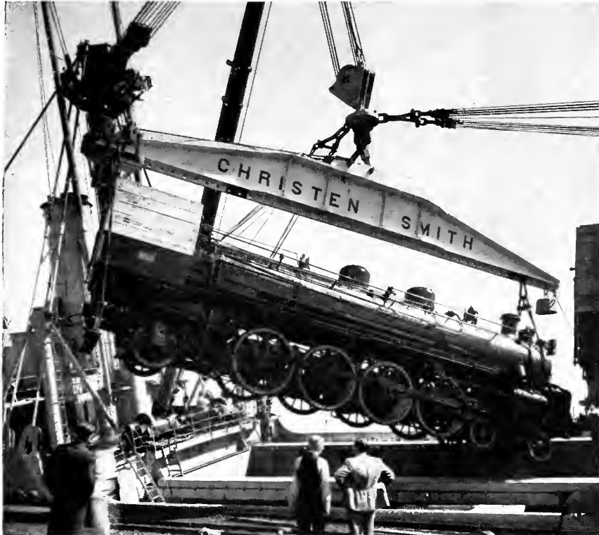
Loading one of seven mountain (4-8-2) type locomotives, for the Chilean State Railways, on board the M. V. Belnor at Baldwin's Eddystone Dock, before the war.
