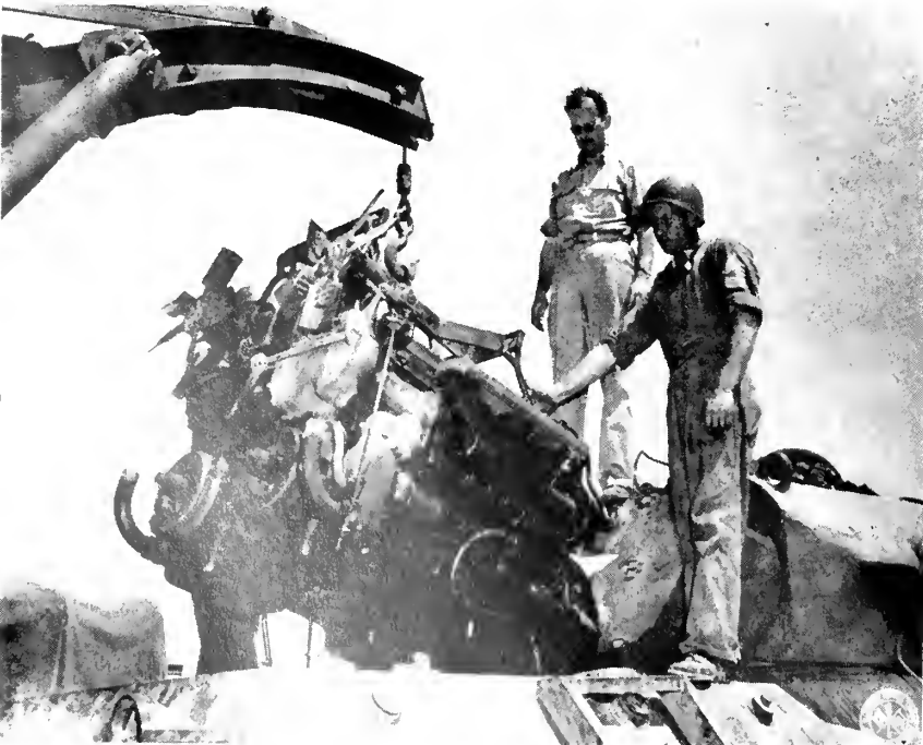
GM diesel motive power for the famed M-4 and M-10 tanks being installed by Army mechanics.
