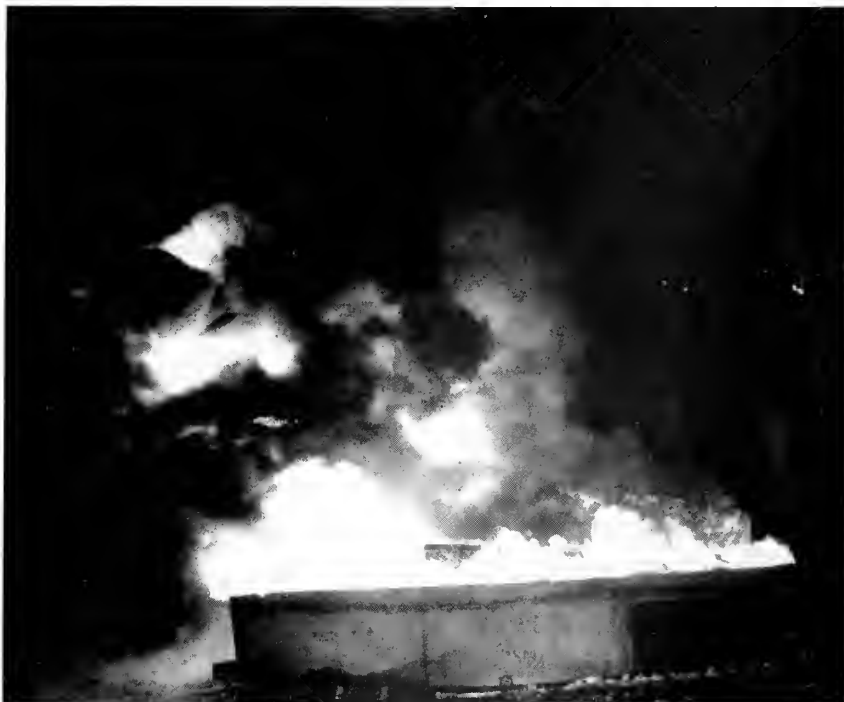
Fire-exposure test on full-size life rafts under way at the Coast Guard Yard, Curtis Bay, Maryland. Rafts have been placed in 30-foot tank previously filled with approximately 1300 gallons of diesel oil.
