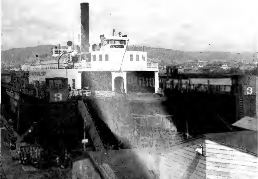
The Richmond-San Rafael auto ferry El Paso on dry-dock recently at Bethlehem Steel Company's Alameda repair yard. Repairs to the vessel included scraping and repainting the under water body, repairing rudder, checking and relining stern bearings and overhauling sea valves.
