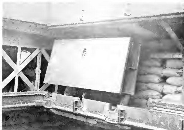
LEFT: Single hinged starboard side cover stowed vertically showing locking device. No strong backs or hatch boards necessary. All tested to open one hatch in less than one minute. Proven after six years of operation. AT RIGHT: Double hinged port side cover stowed vertically.
