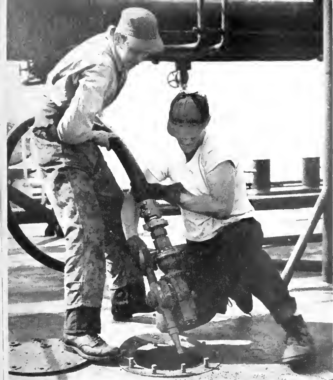
Spraying machine lowered into cargo tanks whirls hot salt water to clean compartment's walls in readiness for another load. Formerly the washing job was done by crewmen who descended into tanks.
