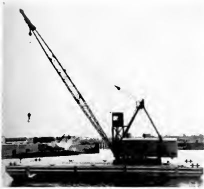
A crane barge complete with crane.
