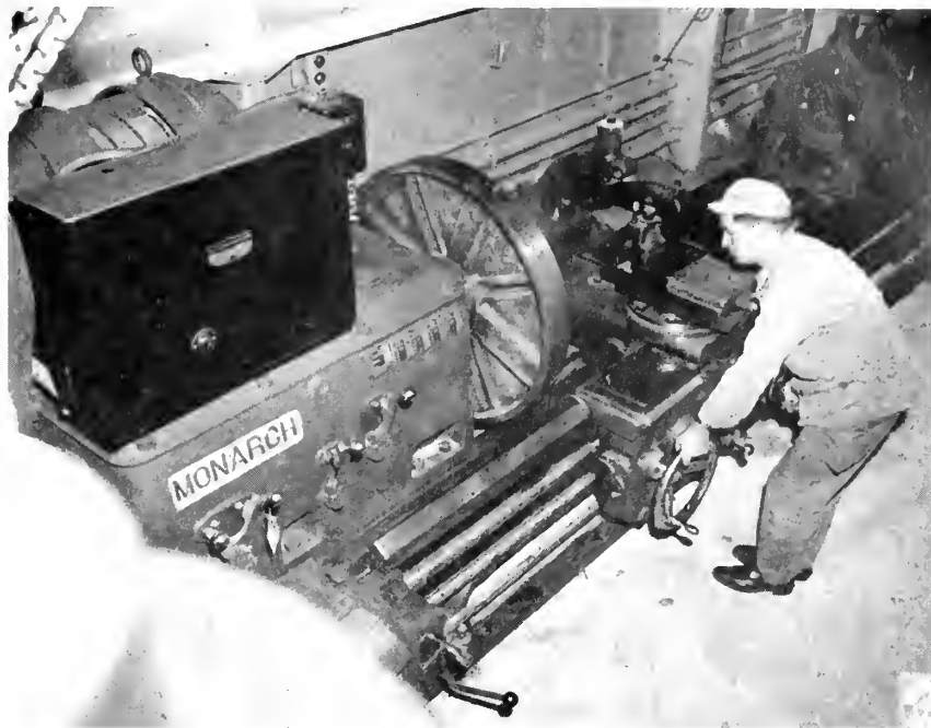
Army marine ship repairman operating 14-ton machine lathe aboard a Transportation Corps vessel operated by the San Francisco Port of Embarkation.
