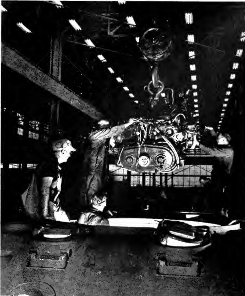
A General Motors diesel engine being installed in an M-4 tank in a Fisher Body plant which produces America's newest type of land fighter.
