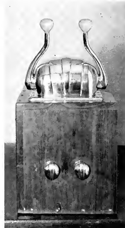
Front view: Showing how double dome appears at control points. One handle may be clutch the other throttle. The small knobs mounted on the face are synchronizing valves, one for each master unit.
