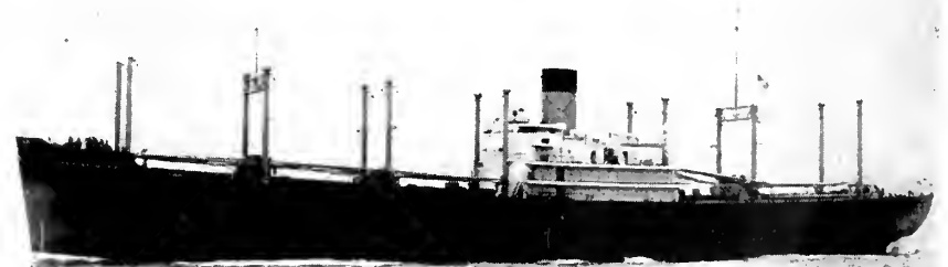
The SS Sea Skimmer , all welded ship of the C3-SA-2 type, recently sailed for New Zealand and Australia under the Matson agency. One of the first peacetime vessels to go into service since the war, the ship, which was built at the Ingalls Shipbuilding Corporation yards in Pascagoula, Miss., was decked out in peacetime paint and featured the new corrugated superstructure which was developed by Ingalls. The Sea Skimmer will carry general cargo and some cargo which requires refrigeration. She also has staterooms for several passengers. She will be used between the West Coast and Down Under on a regular schedule.
