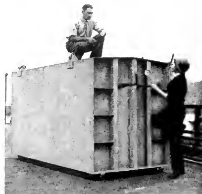
This all-steel hermetically-sealed storage container for a generating unit is getting final check.
