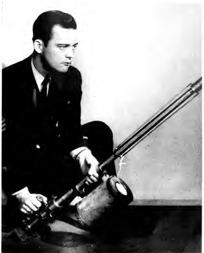
The new Sieg line-throwing gun is demonstrated by its designer, Chief Gunner's mate James E. Sieg. Designed and developed by Sieg under the direction of the Research and Development Division of the U. S. Coast Guard primarily for use by the U. S. Merchant Marine, this gun promises to surpass all previous line-throwing guns in both range and accuracy. (Official Coast Guard photo)
