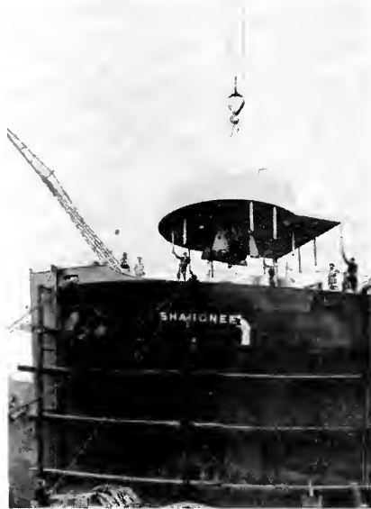
HER GUN PLATFORM REMOVED, her name again on her bow and in trim Socony-Vacuum colors, the veteran tanker Shabonee is converted.
