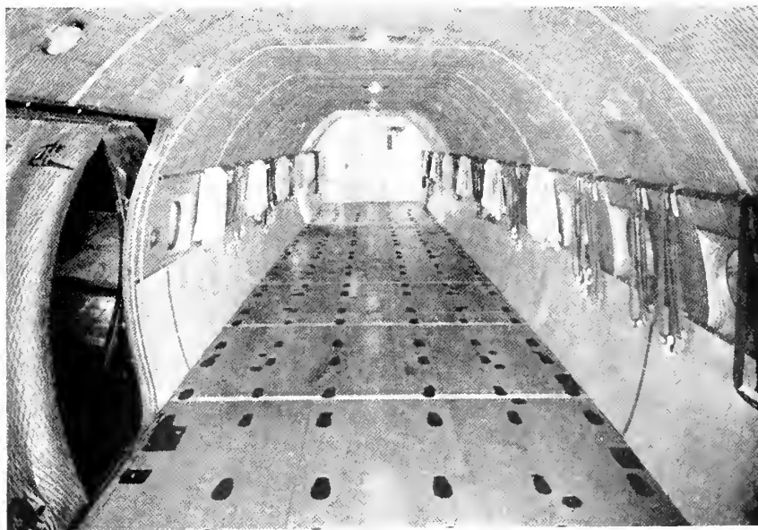
Divested of all military trappings which it had used during service with the Air Transport Command, the first C-54 to be converted at the Martin plant into an air cargo carrier was delivered recently to American Air Lines. Above is the interior of the ship, complete with the necessary tie-downs, cargo lashes and other fittings. The ship stopped off at the new Newark, N. J., Airport and was viewed by thousands. A Martin passenger ramp was taken to Newark for the show and used by the sightseeing throng.
