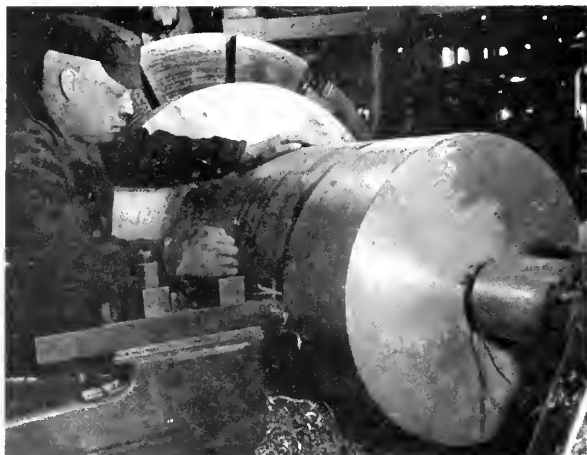
Fig. 8. Coupling journal pin being roughed out. The web fits were machined, finished and ground on this 60" engine lathe. Approximately .035 inch was allowed on the diameter for the shrink fit.
