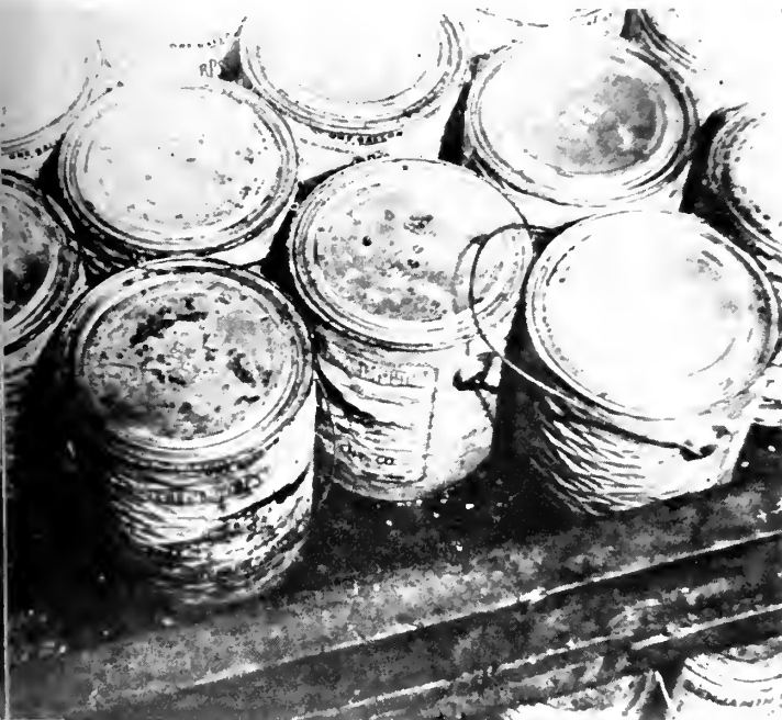
BELOW: A good example of sweat damage—showing canned goods with wrinkled labels and rust spots.
