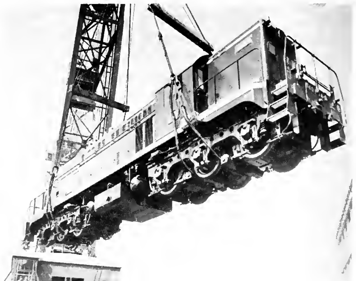
A Baldwin 660-hp. diesel-electric locomotive swinging on board for the trip to Continental France. Recent orders also include 1500-hp. diesel-electrics for French North Africa.
