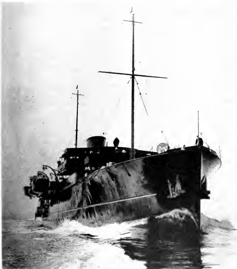
The Williamsburg, built as an ocean-going yacht, has an over-all length of 243' 9"; beam, 36'; mean draft, 14' 6"; maximum draft, 15' 3"; displacement of maximum draft, 1770 tons. Twin propellers are driven by the two 8-cylinder, 1100-hp, 4-cycle General Motors diesel engines. The generator has been replaced with a 3-cylinder G.M. 100-kw diesel generator set. This vessel has been equipped with four guest staterooms, two baths, and an office, bedroom and bath for the President, with adequate accommodations provided for ship's officers and crew and for Secret Service personnel.
