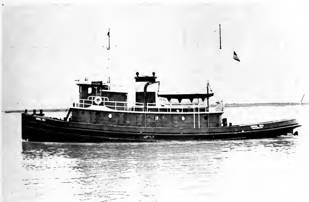
The new 102-foot tug CORAL SEA, built for Interstate Oil Transport Company of Philadelphia by Gulfport Boiler and Welding Works of Port Arthur, Texas, is completely powered by engines built by Cleveland Diesel.
