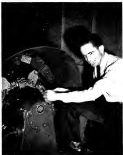
Above: C. D. Singer, port engineer at Seattle, Wash., is pictured inspecting the generator end of a 300-kw Westinghouse turbine-generator aboard a Victory ship in Puget Sound.
