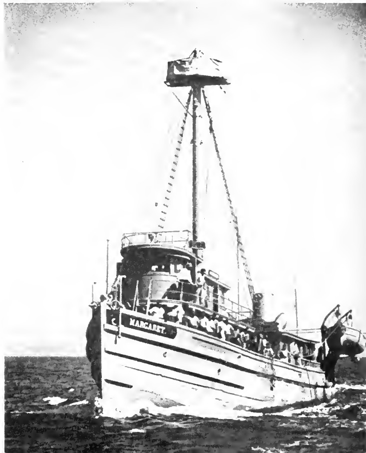
This is the recently modernized Menhaden fishing vessel, the Margaret which is the first of its kind to be powered with a four-cycle, four-valve head, turbo charged Diesel engine.
