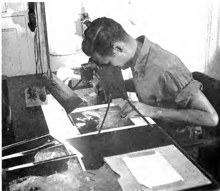
Using a stereoscope on an aerial photographic print, tracing the shoreline and topographic contours.
