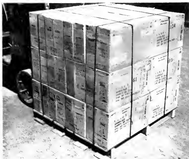
Above: Twenty-four individual containers are handled as one unit by using a pallet and steel strapping.
