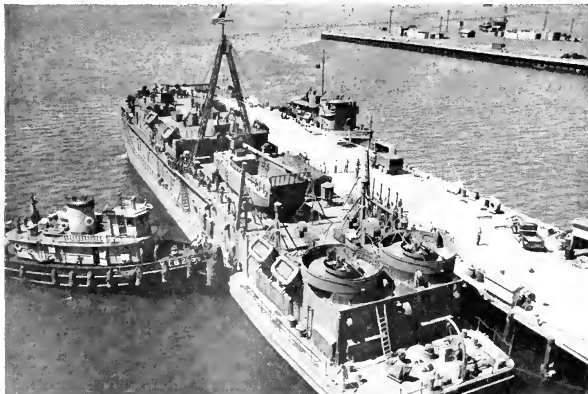
COMPLETED MAINTENANCE BARGE AT BUILDER'S DOCK. Note hinged jib booms stowed just aft of boats and 30-ton boom. Sliding door port side visible under jib boom.
