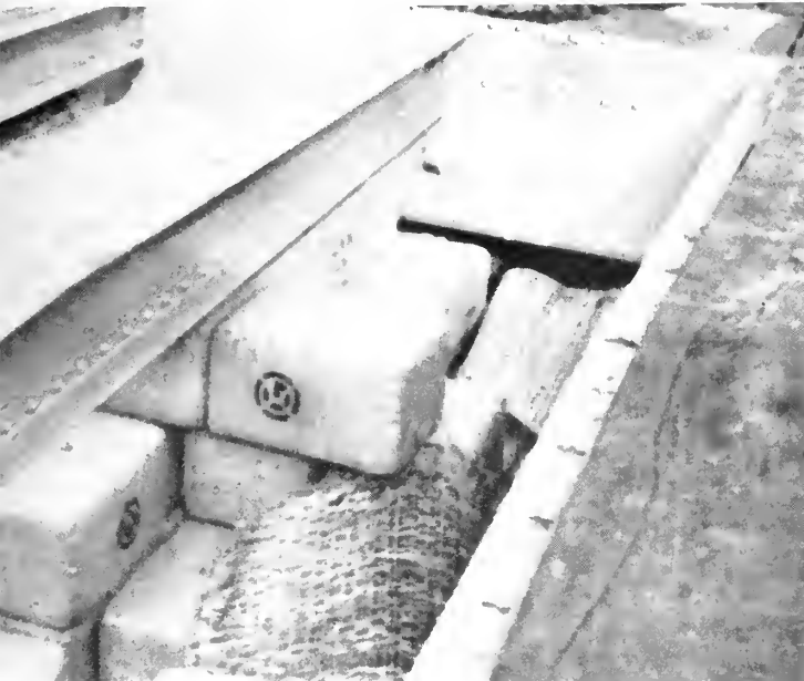
Bags of tobacco after a six weeks voyage on a Cargocaire protected vessel. Notice the dust formed on the steel.
