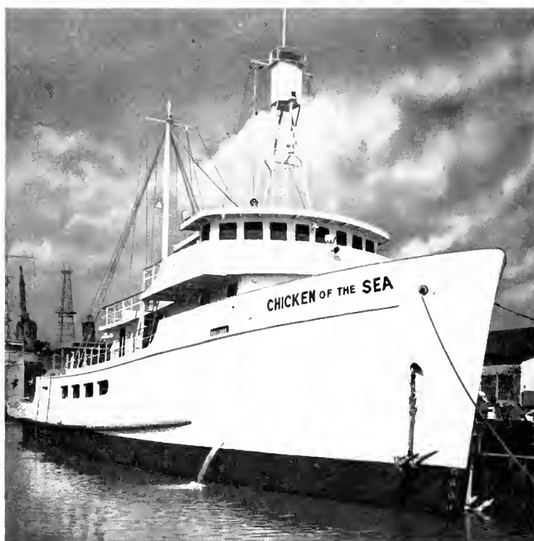
Tuna Clipper Chicken of the Sea shown in new Amercoat dress. New Amercoat antifouling was recently applied below the water line and Amercoat plastic topside finish above. Amercoat anticorrosive primer was used as the base, overall.
