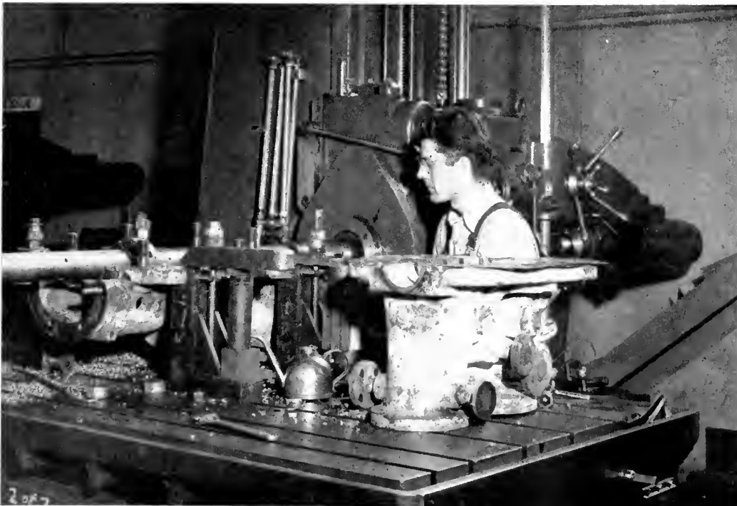
Fig. 9: Machining pump casing on horizontal boring machine.
