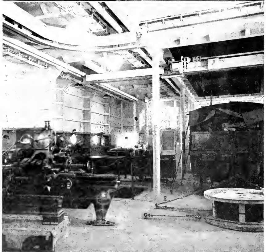
Upper: VIEW IN MAIN DECKHOUSE LOOKING AFT, PORT SIDE. Note 1-ton chain fall lashed on curved spur over small drill press. The short straight spur for No. 4 Port Hold is seen just forward of hoist. Note hand chain pulls for crane interlocks, on crane.
