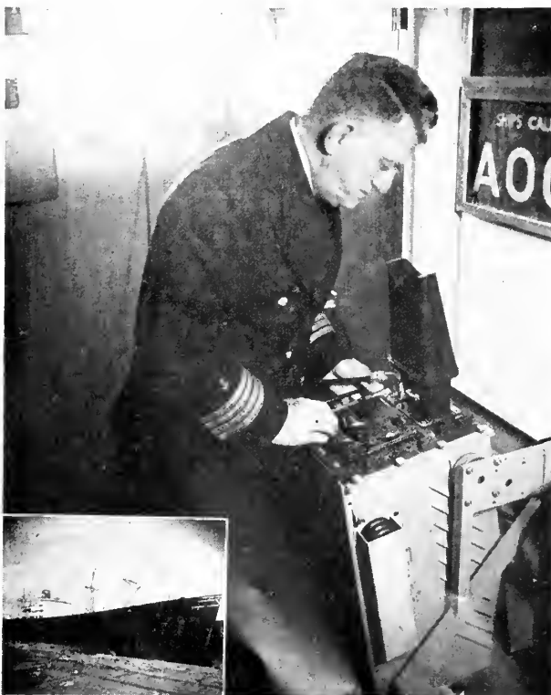
Captain E. R. Callaway, of the Waterman liner John B. Waterman, examines RCA loran receiver which his vessel used to complete first loran-guided crossing of the Pacific. (Inset) The John B. Waterman at the end of a 20,000-mile voyage, completed in 127 days.
