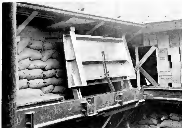
LEFT: Single hinged starboard side cover stowed vertically showing locking device. No strong backs or hatch boards necessary. All tested to open one hatch in less than one minute. Proven after six years of operation. AT RIGHT: Double hinged port side cover stowed vertically.
