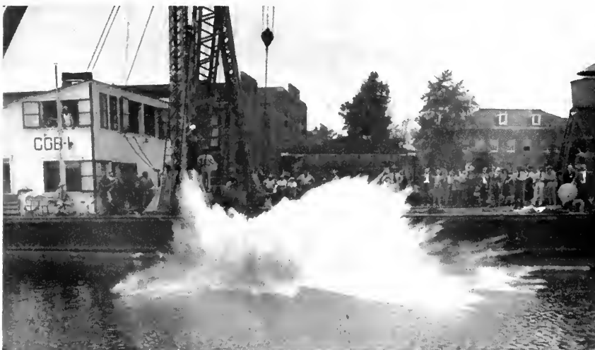
Hidden from view by the spray, this raft hit the water endwise after a 45-foot drop.
