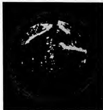
Radiomarine Corp.'s new shipboard radar dial showing the 12" PPI scope picture.
