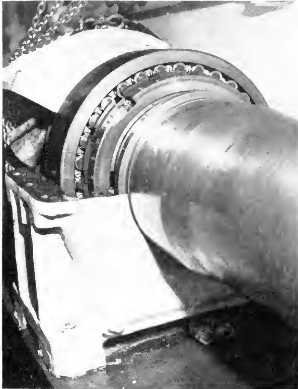
One of the spherical roller bearings on the USS LeJeune, with top housing removed to permit inspection.
