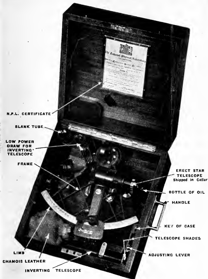
Fig. 3: A "diamond frame" micrometer sextant stowed in its case. Note the position of the index bar (about halfway along the arc) and the erect telescope shipped in position.
