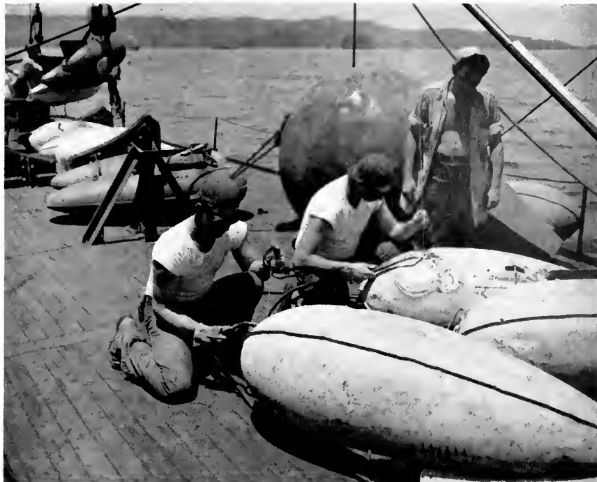
U. S. S. Sumner. Repairing improvised drag buoys made from belly tanks. These buoys support the wire drag net, which is of a fixed depth. This drag net is towed slowly through the water of a harbor to make sure that the harbor is free of pinnacles or other hazards to navigation. (Official U. S. Navy photo)
