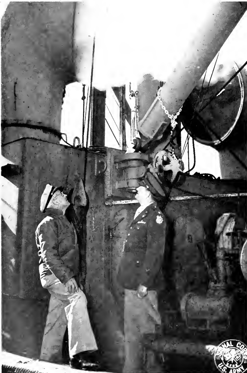
Using Air-mover in port ventilator to remove gases from the hold —steam used as ejecting power.
