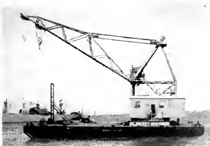
A 60-ton crane barge on the way to a harbor job.
