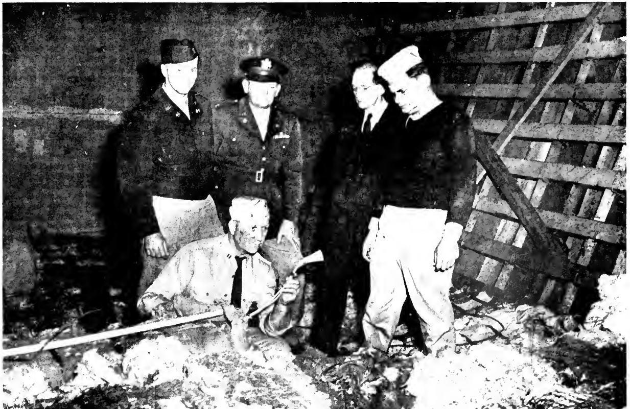
Lt. Bender, Major Christian, Mr. Culp and Commander Layman watching Lt. Peterson prepare to ignite cotton cargo in No. 5 lower hold.
