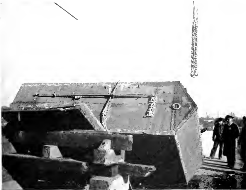
After strafing, the Royal Marine Equipment Co. (New York City) wood raft is still a dependable life-saving unit, as the cork buoyancy unit is practically intact.
