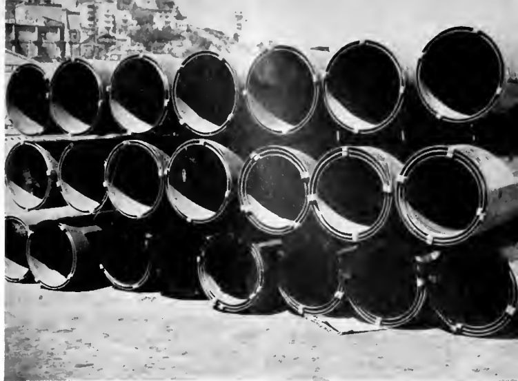
Here are 20, 22 and 24 inch oil line pipes for Arabia. The sections are 30 feet long and are nested and spot-welded to save cargo space.
