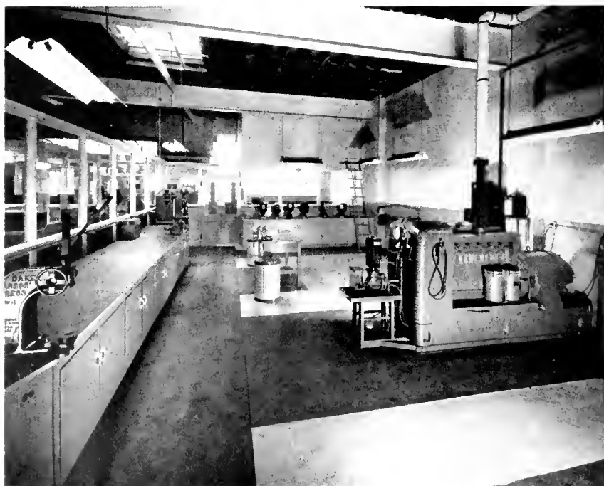
Interior view of the Marquette Governor Service and Training Station, New York shop. Similar shops are in New Orleans, Los Angeles and Emeryville, California. At the right a reconditioned governor is being tested on a diesel engine.
