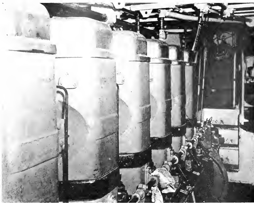
Enterprise D.M.G.-6 400-hp main propulsion unit on the shrimp boat Sovereign.
