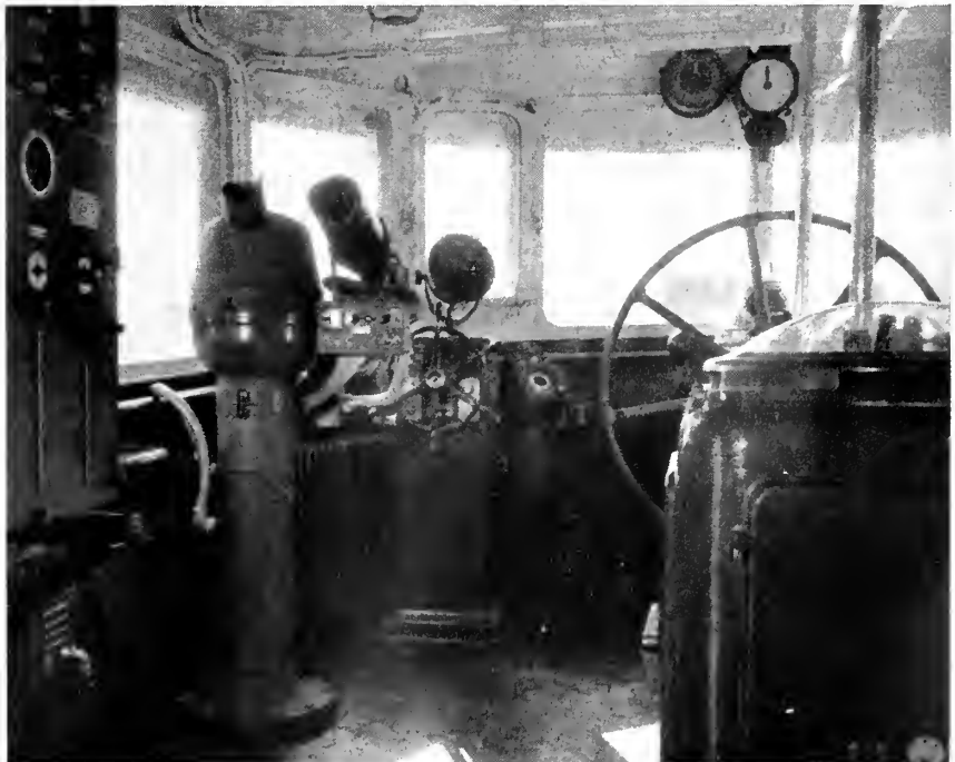
Array of new navigation instruments seen in this photo are undergoing service tests on the "Floating Laboratory." These instruments include automatic steering apparatus, radar devices, and other equipment navigators dream about.
