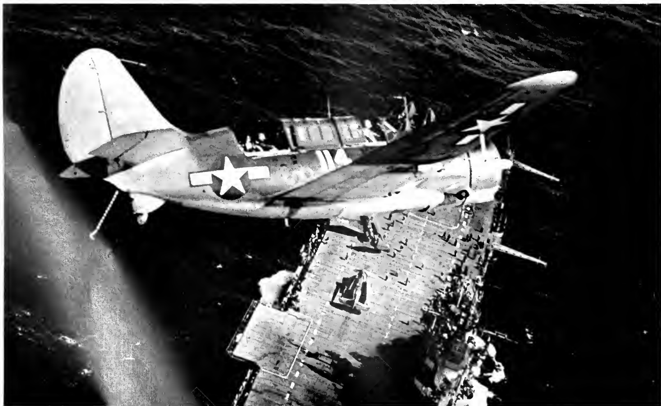
Jutting from the carrier's midsection is the deck-edge elevator by which planes can be shuttled between hangar and flight deck with dispatch. (Official U. S. Navy Photo)
