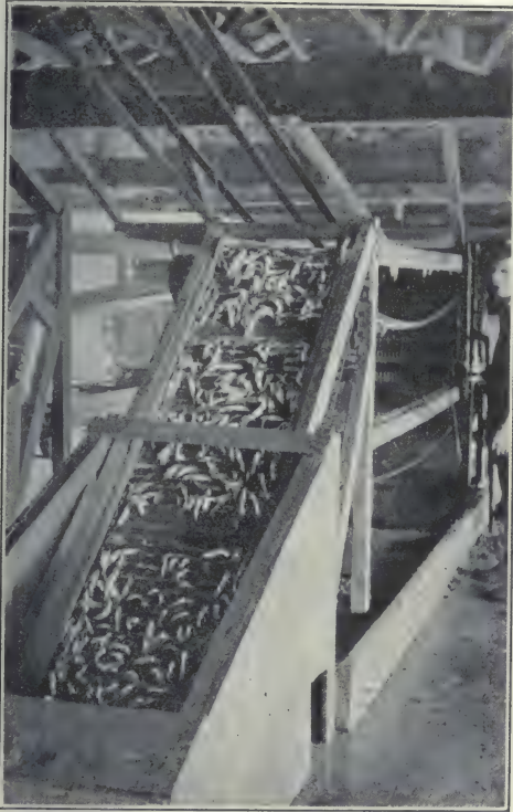
Fig. 3—Showing the Hopper or Endless Belt Arrangement, which Carries the Fish from the Brine Tanks to the Flakes.
